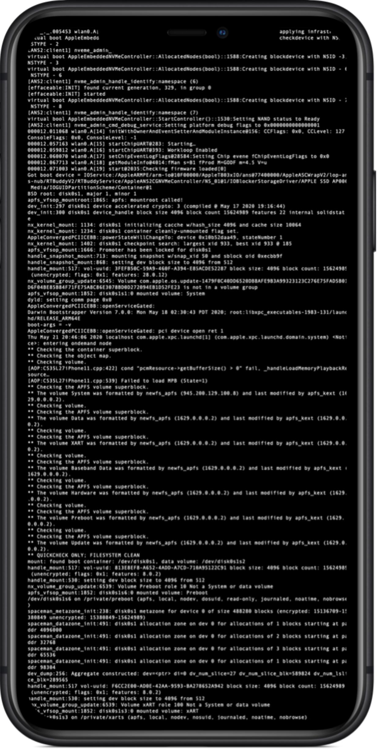
A black smartphone is shown from a top-down perspective, displaying a terminal window with a black background and white text. The text is a detailed log of a boot process, showing various kernel messages, device detections, and configuration steps. Key terms visible in the log include "AppleEmbedded", "NVMeController", "APL", "APFS", "APFS\_XART", and "spaceman". The log ends with a "nobrowse" command at the bottom.
